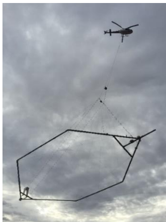
Helicopter AEM system with an antenna frame.
